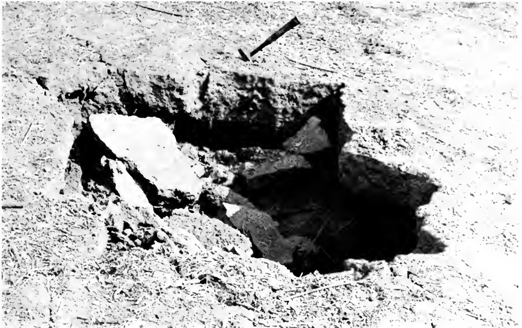
Photo 1. Crater resulting from consolidation of soft soil by a small dynamite blast during seismic refraction survey.
